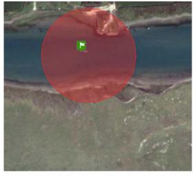
in SOS capabilities and these can be directed to any given e-mail or smsaddress. Users can also set up geo-fences around specific areas and if the vessel were to enter of leave these areas, notification can be sent. This facility can be very useful in the case of moorings etc. Finally the Succorfish SC2 system can be used to notify the vessel owner when the on-board batteries run low and in future other remote monitoring will be added.
